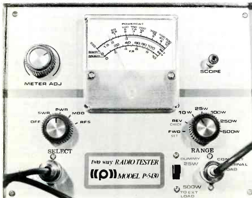
Power output during this test is only 0.6 watt. Is the transmitter defective? No, a mistake has been made in connecting the test equipment. The error will be explained next month in Part 2.
