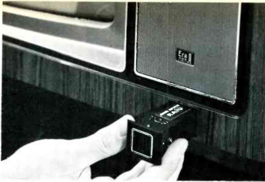
Fig. 3 Several Admiral "Era II Limited" models have provisions for adding a remote amplifier at any time. The plug-in unit, plus the portable remote hand unit, provide full remote operation.
