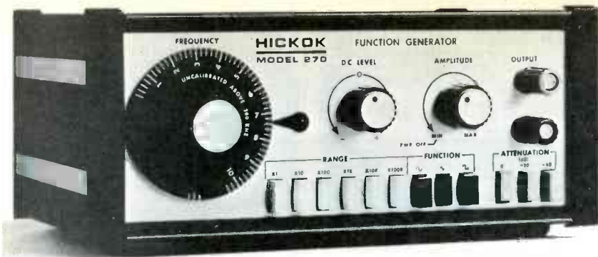
Fig. 5 The Hickok Model 270 Function Generator not only produces sine, triangular, and square waves between 1 Hz and 1 MHz, but by use of some connections in the rear, also can generate sawteeth and pulses.
