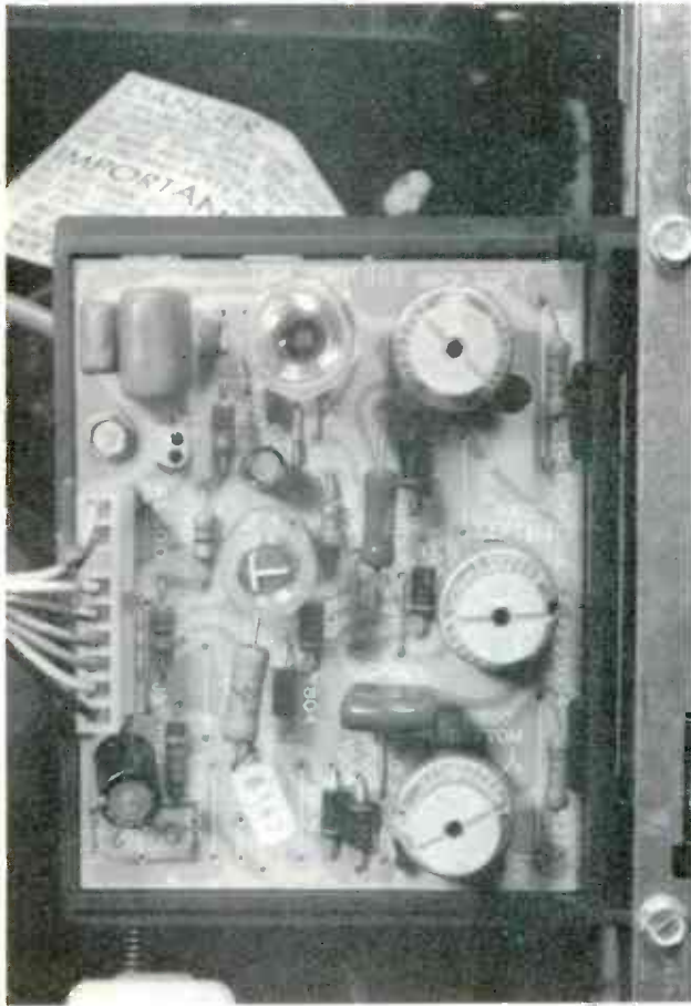
Picture 15 The dynamic-convergence board is located in the upper-right corner of the chassis frame. Only one coil and three controls are adjustable.
