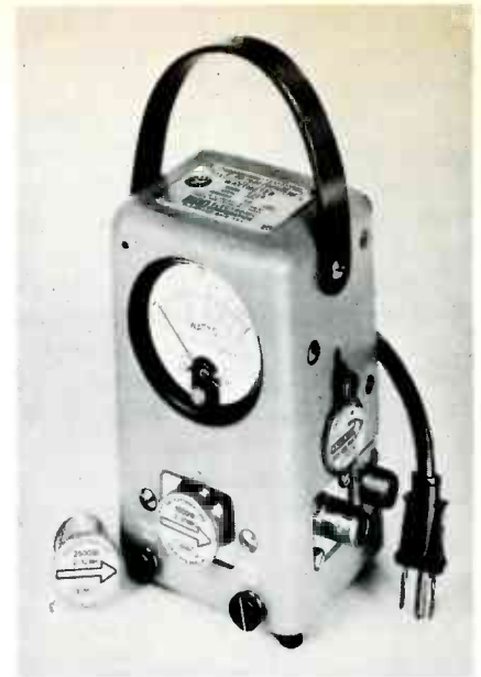
Fig. 3 Bird Electronics offers several types of power wattmeters. Although this kind does not measure SWR directly, it measures both forward and reverse power flow. If the reverse power is less than 5% of the forward, the SWR is satisfactory.
