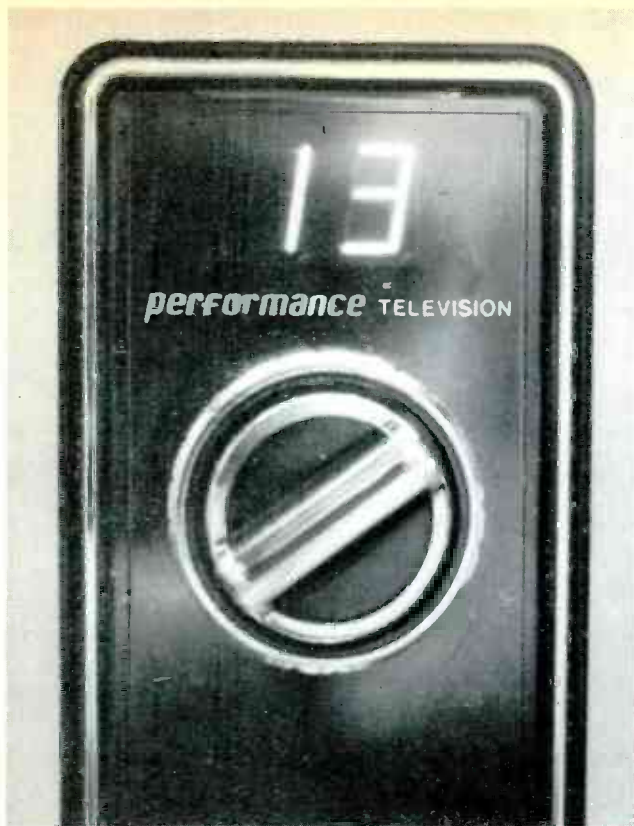
Picture 2 Turn on the power, and the ½-inch channel numbers light up in orange. All 12 VHF and 69 UHF channels are displayed on the two-character 7-segment glow-discharge type of readout. The position between 2 and 13 of the VHF knob at the top causes the same display to show the UHF channel which is selected. The lower knob is detented for every UHF channel, and it can't turn beyond 14 and 83. When I first tried it, the mechanism worked excellently, and I liked it after I became familiar with the action. But the operation felt strange and different because the numbers do not move sideways (as older models did where the numbers were on a drum), and there was no vibration, except for the detenting.
