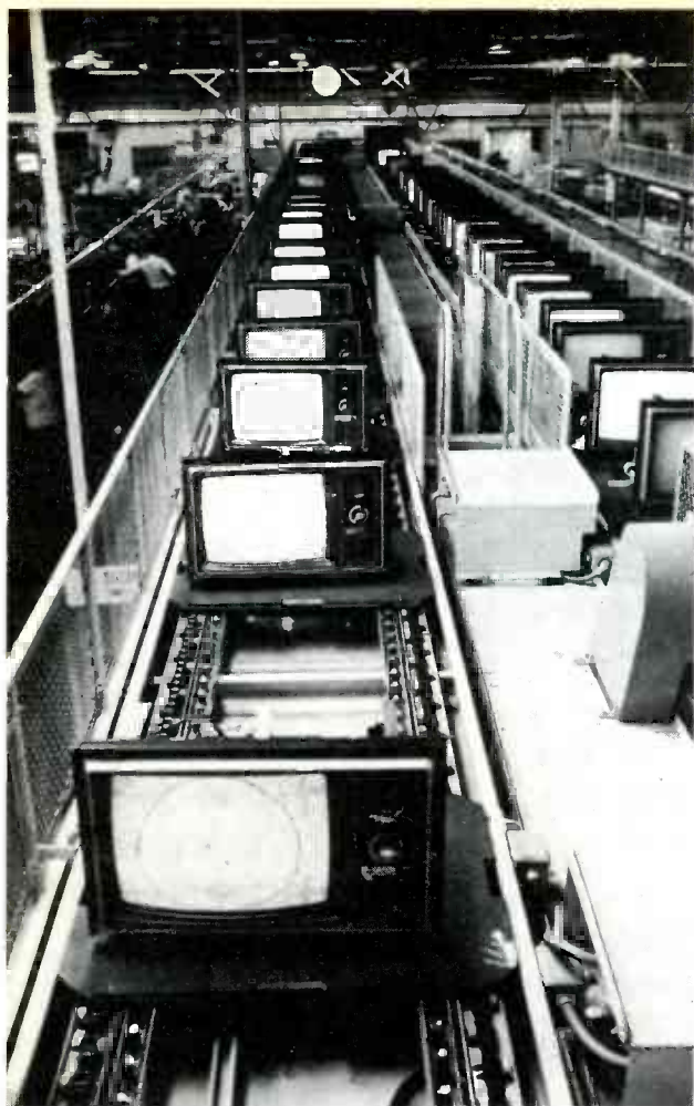
Fig. 7 New Quasar color receivers take a slow ride during their time test before final testing.
