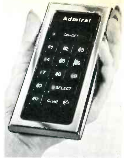
Fig. 4 The Admiral remote-control transmitter requires only a 9-volt battery to become operational.
