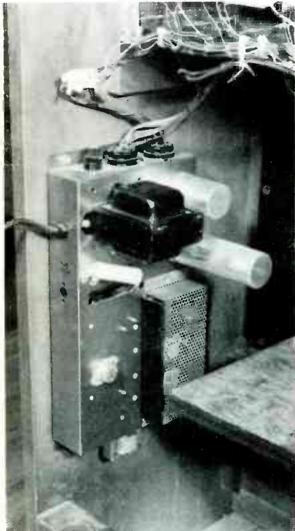
Fig. 4 These points of a tube-type amplifier are best for the "buzz" or audio-source tests. With signal-injection checks, you usually start at the input of the output tubes or transistors and work back toward the low-level stages.
